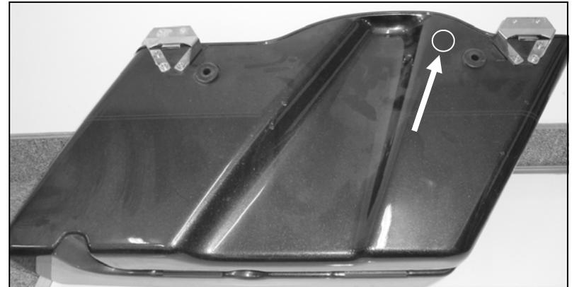
The white circle in the picture above is where a 3/4" (19mm) hole will be drilled. This hole is where the supplied Hogtunes rubber grommet will go, and allow the speaker wire for the lid to pass into the saddlebag.
