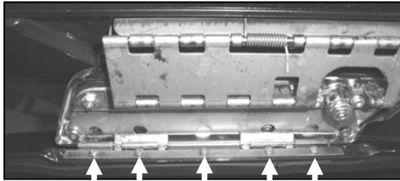
With the flap off, fold the factory lid all the way over, exposing the 5 screws highlighted above by white arrows. When these are removed, the factory lid will be free from the saddlebag. These screws will be used to install the new lid so keep them handy. With the factory lid off the bike, you will see a metal “strip” between the rubber gasket and the lid itself that the screws just removed threaded into. This metal strip must be removed as it will be used to install the new lid.
