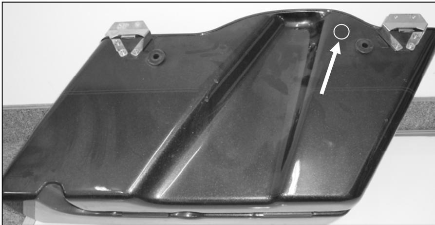
The white circle in the picture above is where a 3/4" (19mm) hole will be drilled. This hole is where the supplied Hogtunes rubber grommet will go, and allow the speaker wire for the lid to pass into the saddlebag.
