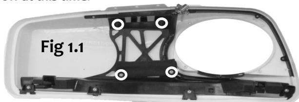
Locate the metal plate with the passive crossover installed and sit it in place so it is oriented as shown in Fig 1.2. There is a specific brake side and clutch side, so put the one in so all 4 holes in the plate line up to the holes in the lid. Re-install the 4 screws noting that the tether will sit on top of the crossovers mounting plate.
