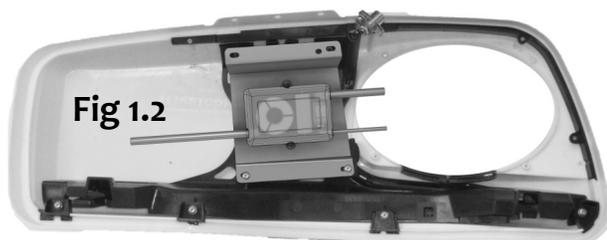
Locate one of the tweeter assemblies (they are the same for brake and clutch side) You will see a groove on the tweeter assembly that mates to the lid. Locate the black gummy material that came in the kit and take one strip, roll it in your fingers so its close to uniform thickness and apply across entire groove highlighted by arrows in Fig 1.4 on next page.
