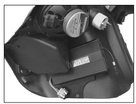
Step 3) Clean area on inner fairing where other half of hook and loop adhesive will go. The bolts that hold the turn signals in place will secure the plate even though the adhesive does most of the work. Plug the supplied power harness extension into amp and follow amplifier manual for wiring instructions.
