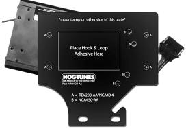
Step 2) Put the plate over the amp as shown above and reinstall 4 screws into <u>holes marked "B"</u>. Apply 1 side of hook and loop in area shown on plate.
