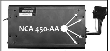
Step 1) Turn the NCA 450-AA over and remove the 4 screws (shown above) on the power connector side of the amplifier
