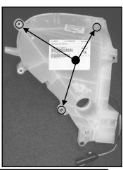
Note: Brake Side Shown, But Fastener Location Is Same For Clutch Side
