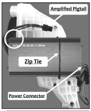
Fig1.4 Amp Correctly Placed
