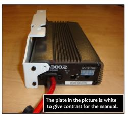
Step #6: Slip the mounting plate over the amp as shown and reinstall the 2 screws into the front, and 2 screws into the back of the amp.
