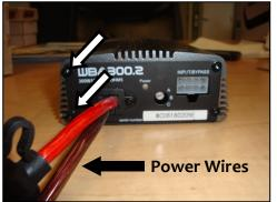
Step #5: For this installation, we will refer to the power "end" of the amp as the front. Remove the 2 small allen head fasteners highlighted by the white arrows. Also remove the 2 screws on the back end of the amp, directly opposite the first 2 screws just removed.
