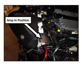
Step #7: The holes on the top of the plate mate with the screw holes on the top of the speaker cabinet (bolt holes in Fig 1.2) Holding the amp in position, slide the cabinet/amp into position noting that the amp plate sits over TOP of the factory metal plate. When correctly in place, the factory screws will go
